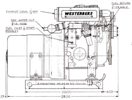
**DESIGN:** Four pole revolving armature, inherently regulated, self limiting, rectifier excited, A.C. slip rings, single bearing design.
